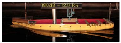
Still Water Resistance and Propulsion Tests
