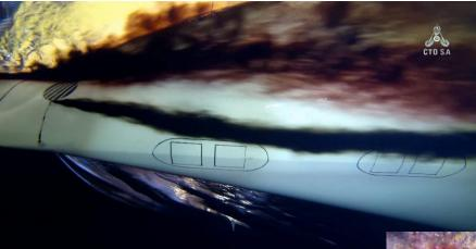
Flow Visualization in way of two alternative Sensor Positions by means of Underwater Camera Footage
